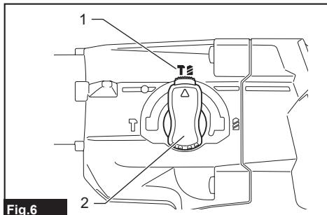
Fig.6 ▶ 1. Rotation with hammering 2. Action mode changing knob
